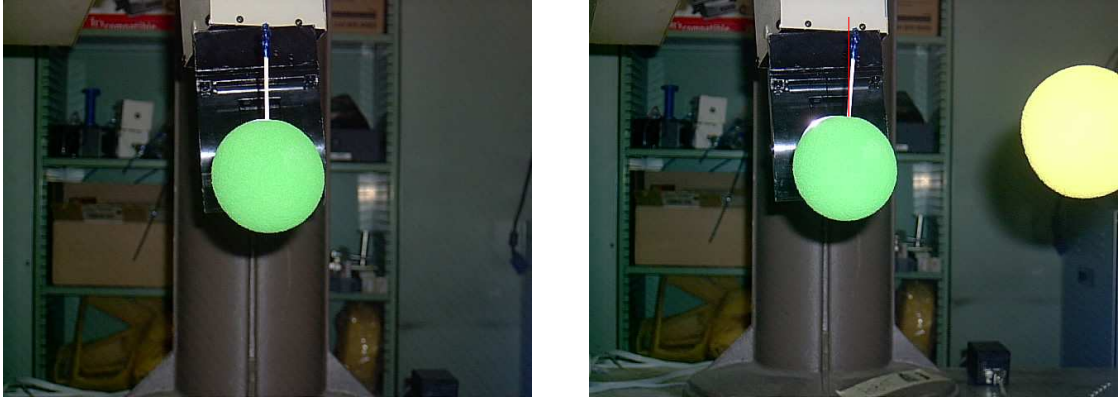
Figure 5.24. Beginning and Ending Configurations of a Robot Finger Following a Lie Bracket Motion to Effect a -5^\circ Rotation
