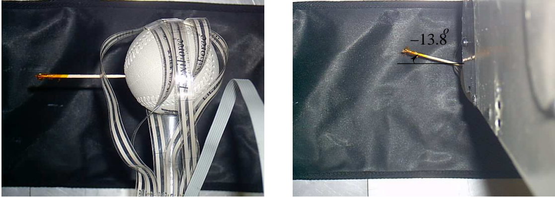
Figure 5.4. Mechanical Coupling of the Wrist Joints. When joint five is commanded to rotate, joint six passively rotates.
