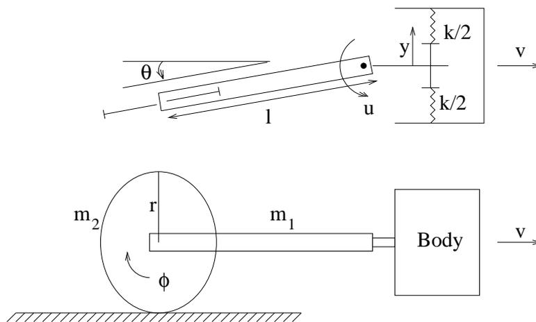
Figure 1. Classical shimmying wheel model.
