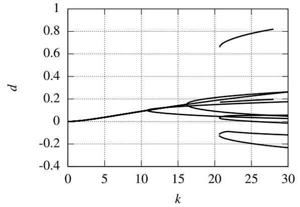
Fig. 7. Bifurcation diagram for robot number six in a seven-robot system.
