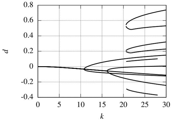
Fig. 4. Bifurcation diagram for robot number three in a seven-robot system.
