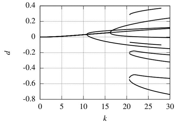
Fig. 6. Bifurcation diagram for robot number five in a seven-robot system.
