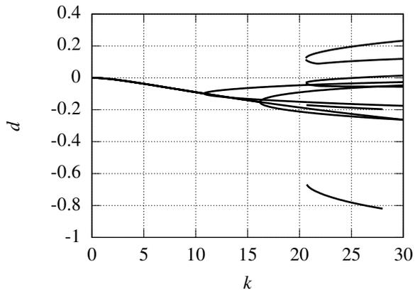
Fig. 3. Bifurcation diagram for robot number two in a seven-robot system.
