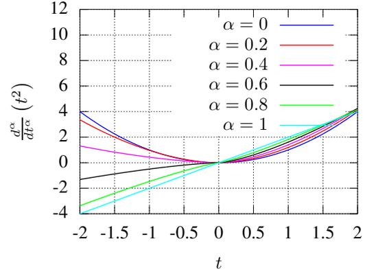
Fig. 5. Fractional-order derivatives for  $f(t) = t^2$  for various orders between 0 and 1. Note that the zeroth derivative is the parabola, the first derivative the expected straight line and the fractional derivatives between these two vary in a reasonably expected manner.
