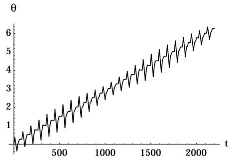
**Figure 5.10.** Hexapod orientation during execution of path seen in Figure 5.9.
