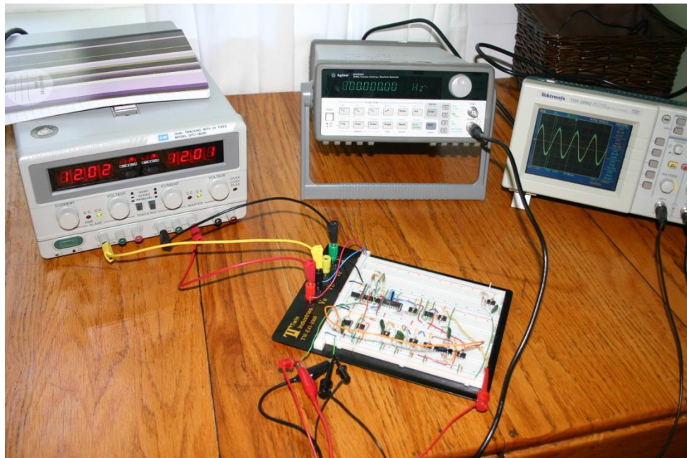
Figure 6.2: Photograph of the experimental setup for the function generator testing performed on the AO controller circuit.
