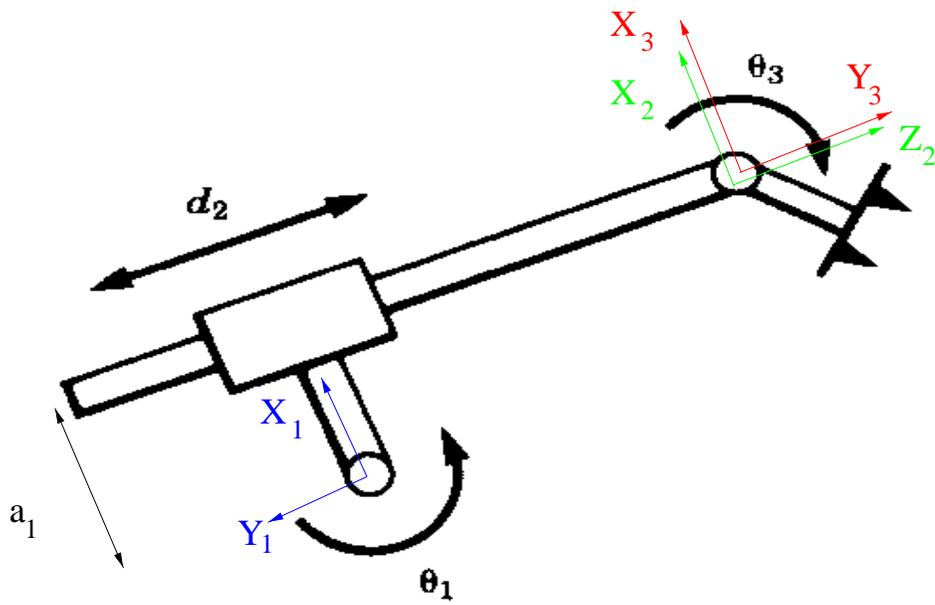
Figure 2. Link frame assignments for problem 2.
