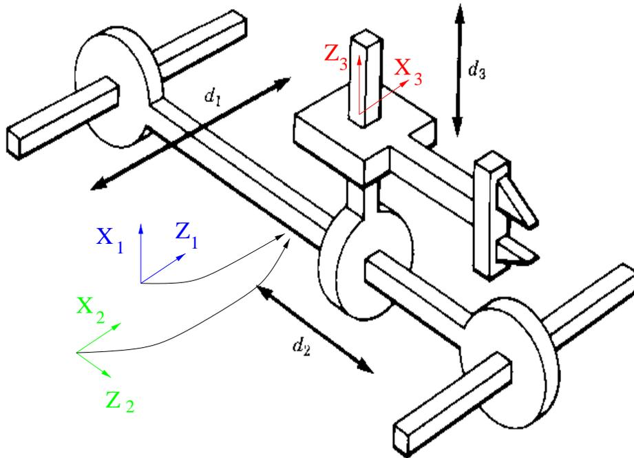
**Figure 3.** Link frame assignments for problem 3.
