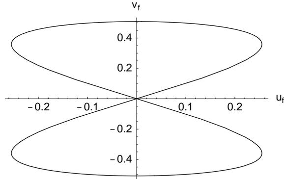
**Figure 5.16.** Trajectories for finger contact coordinates: sinusoidal inputs.
