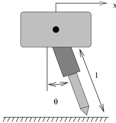
**Figure 4.1.** Kinematic leg.
