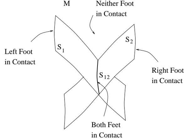
**Figure 2.2.** Schematic view of the configuration manifold structure of a biped robot.
