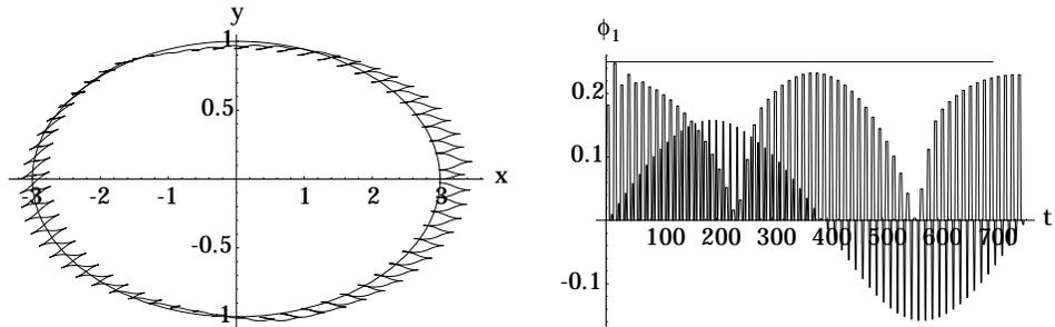
**Figure 5.8.** Elliptical trajectory and stability criterion for the hexapod robot taking smaller steps.
