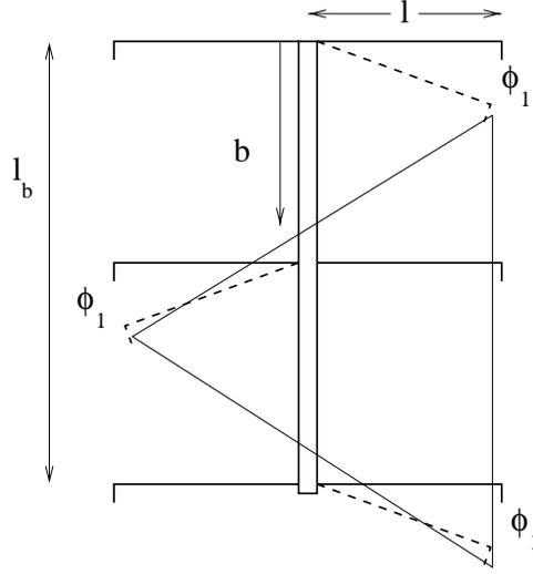
**Figure 5.5.** Stability margin for hexapod tripod gait.
