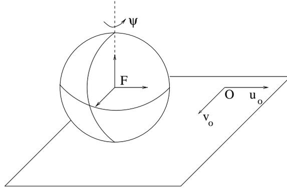
**Figure 5.14.** Spherical finger rolling on a plane.
